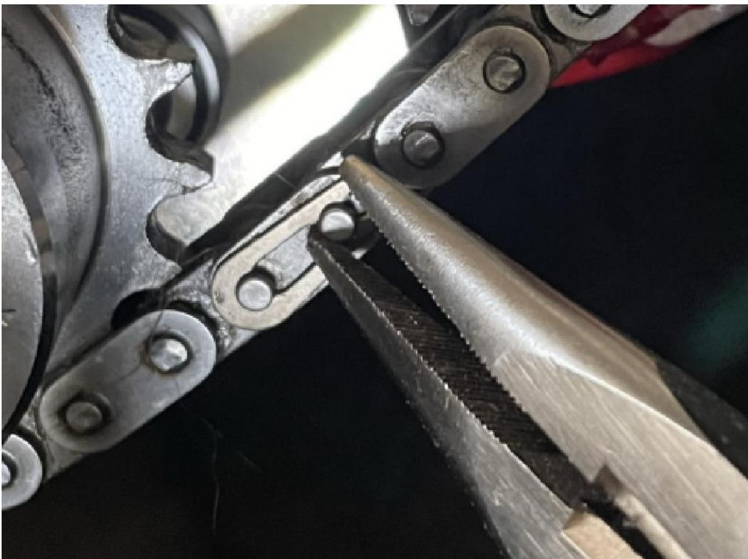
[ ] Remove the retaining clip from the retaining plate.
