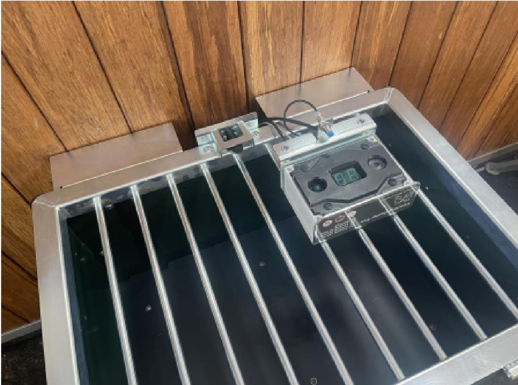
[ ] Unscrew the 4 bolts from the front of the controller housing with a Phillips screwdriver. The bolts are secured to the front of the housing. These can only be unscrewed, but not removed.
