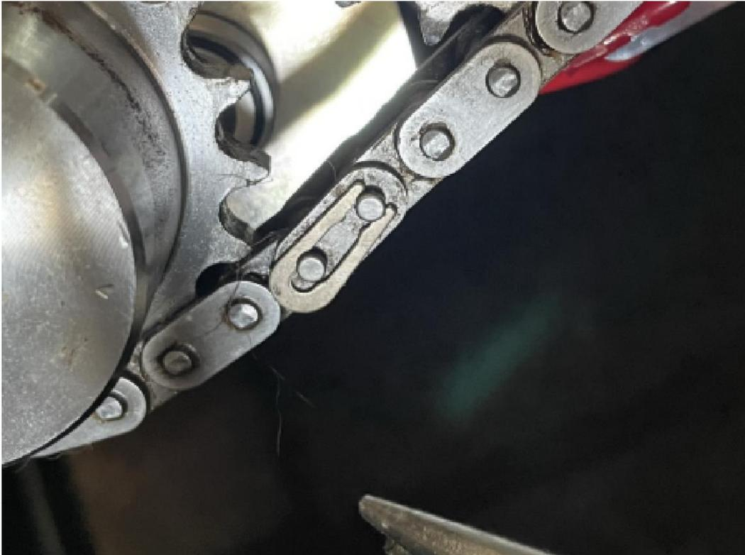
[ ] Remove the retaining plate from the coupling part.
