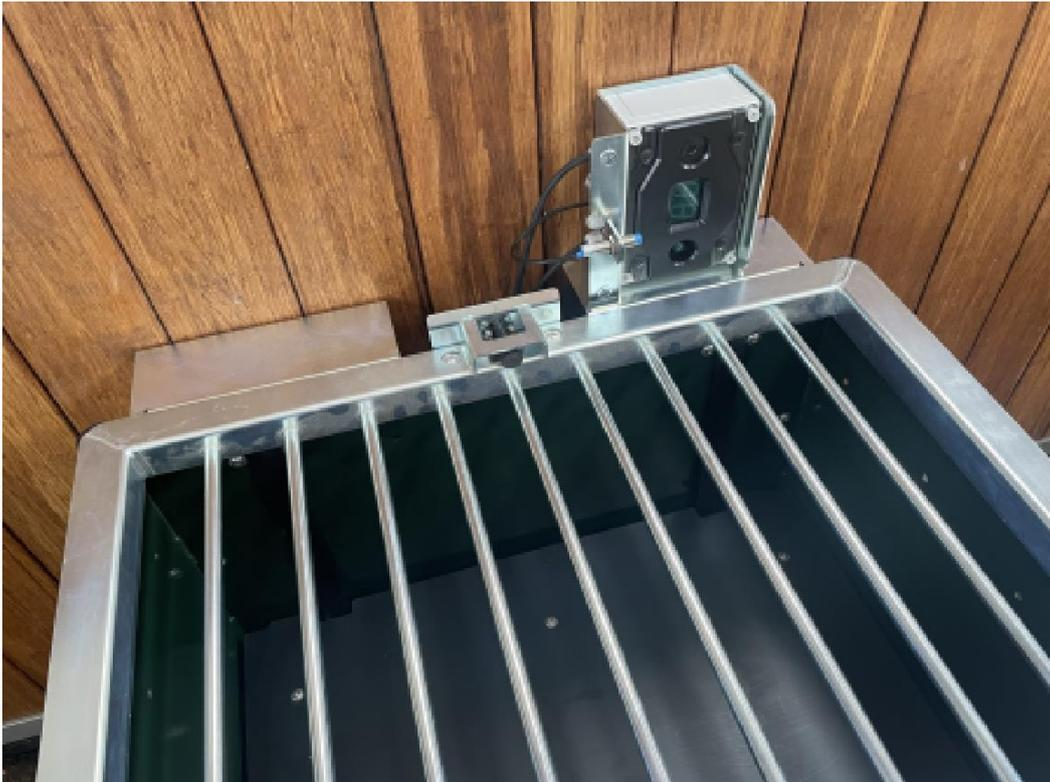
[ ] Open the grid. To prevent the grid from touching the grid sensor, it may be necessary to lift the control slightly while opening the grid.
