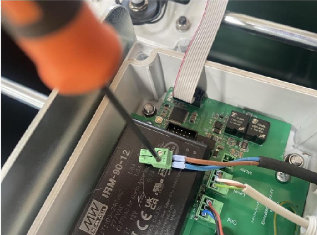
[ ] Remove the wires from the plug.
