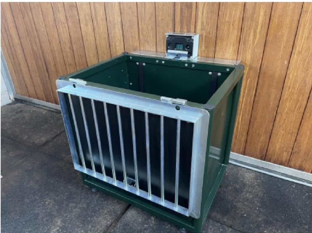
[ ] Remove the two allen bolts holding the controller with a 5mm allen key.
