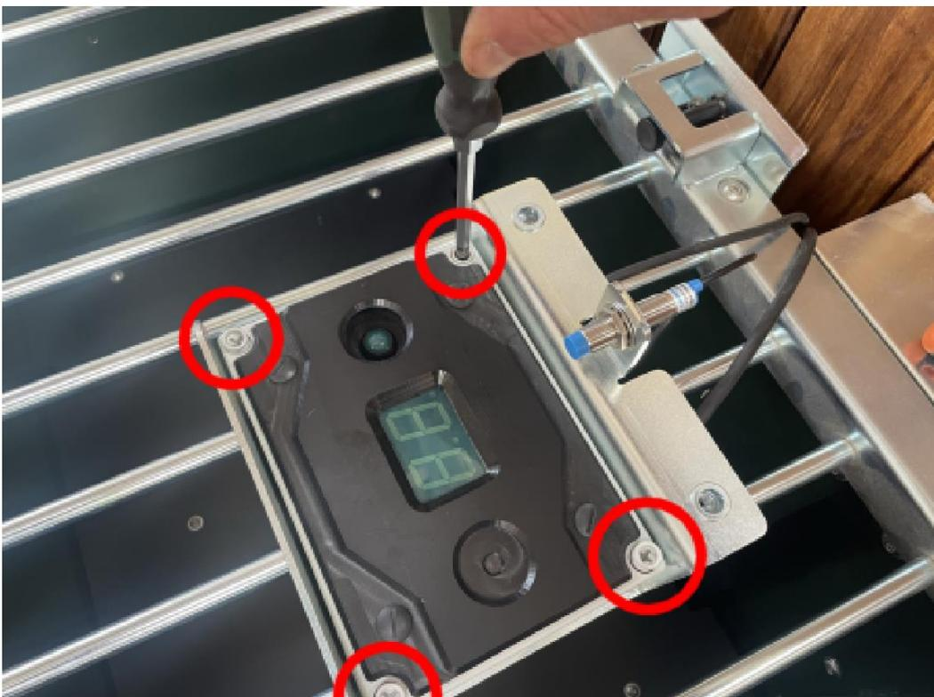
**WARNING:** If the nuts are tightened too hard, the silicone gasket between the front and back of the housing will be crushed and the two parts will no longer be watertight. Moisture can then condense in the housing, causing the controller to malfunction.
