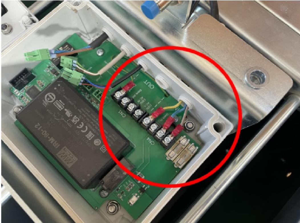
[ ] Unscrew the three connections of the power cord on connector CN4.
