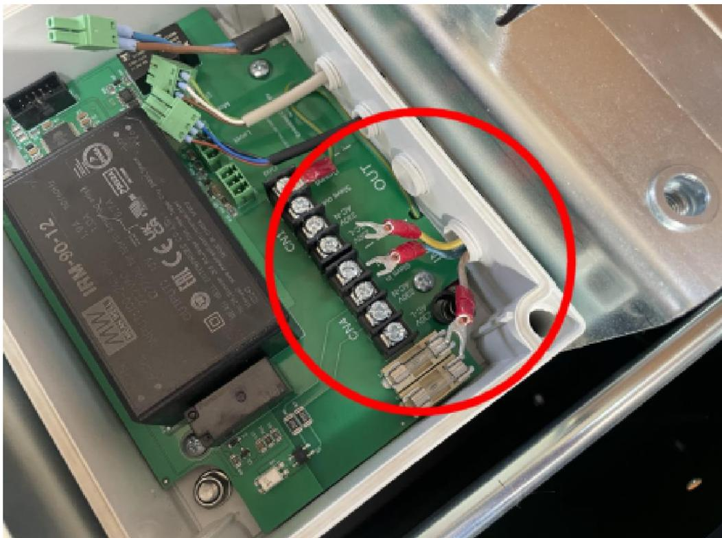
[ ] Unscrew the ground connection of the connector CN1.
