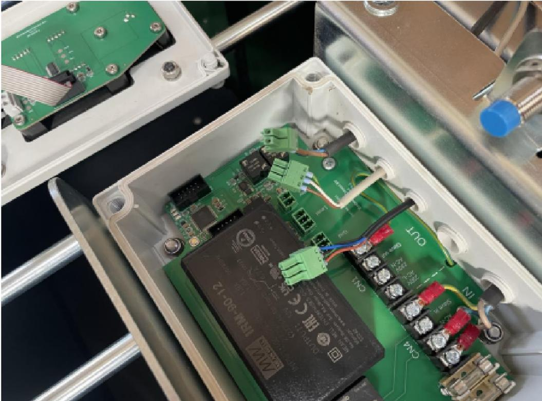
[ ] Remove the strain relief from the cable.
