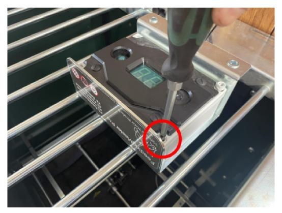
[ ] Place the controller back on the right mounting bracket.
