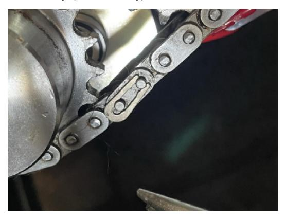
[ ] Remove the retaining plate from the coupling part.
