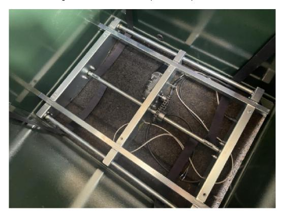
[ ] Slide the motor cable under the rear wall of the FeedingMaster. Pick up the cable through the hole between the mounting brackets and gently pull it up.
