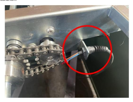
[ ] Remove the motor cable from the strain relief. Place the loosened part of the strain relief back half a turn so that it is not forgotten later.
