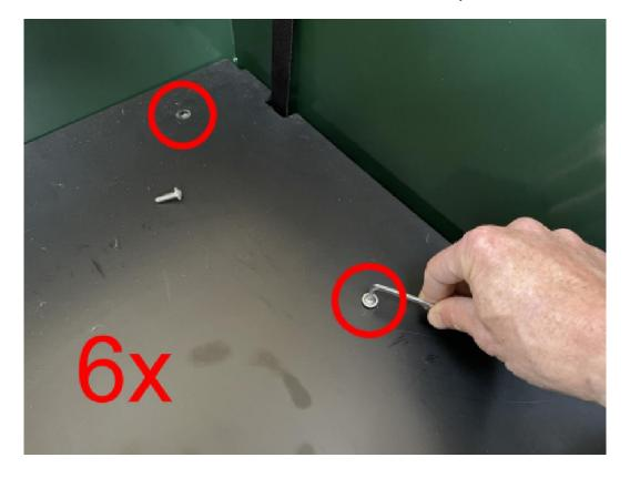
[ ] Remove the feed floor from the FeedingMaster Pro.
