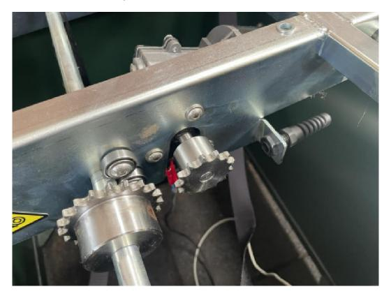
[ ] Loosen the three bolts that secure the motor to the feed mechanism. Use a 4mm allen key for this.
