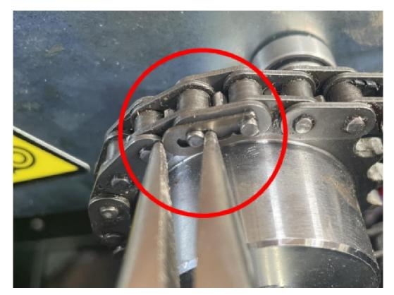
[ ] Press it with needle-nose pliers.
