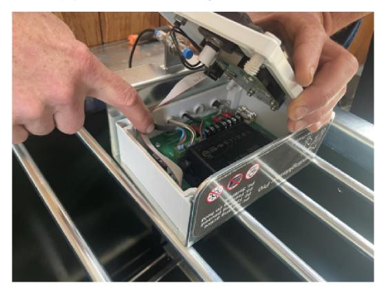
[ ] Place the front of the housing on the controller housing. Check that there are no wires between the parts and that the front of the housing rests neatly on the back of the housing.
