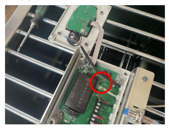
[ ] Loosen the terminals of the plug with a small flat screwdriver.
