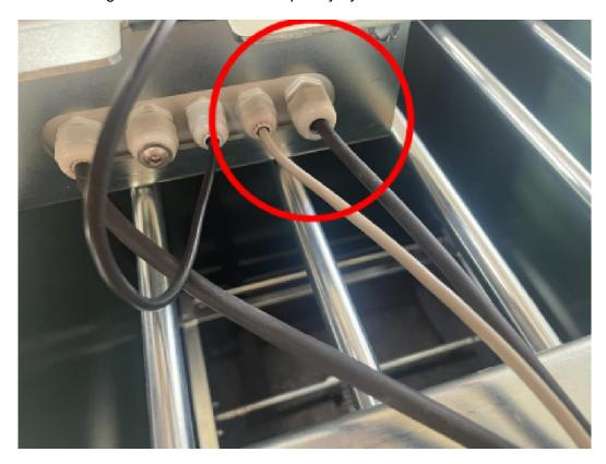
[ ] Place the front of the housing above the controller housing. Carefully press the connection cable of the display into the corner of the housing.
