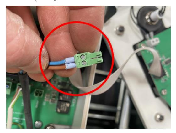
**WARNING**: Check the wires again. If they are connected the wrong way round, the feed floor will move the wrong way around when the FeedingMaster Pro is switched on and the height sensor will be permanently damaged.
