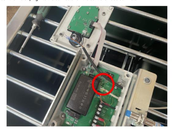
[ ] Gently pull the motor cable out of the strain relief until it is as short as possible but not yet under tension. Tighten the strain relief completely by hand.
