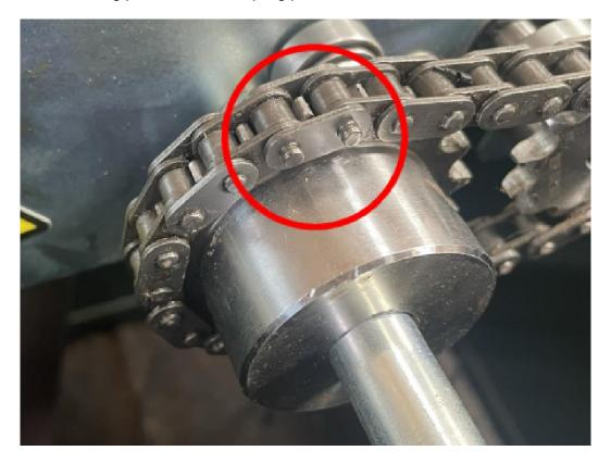
[ ] Place the retaining clip over the retaining plate.
