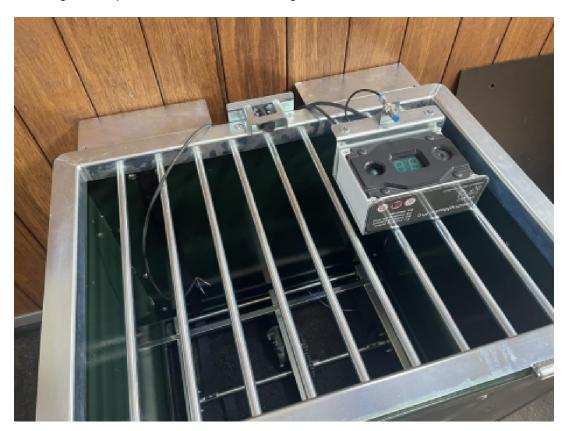
[ ] Unscrew the nut in the front of the controller housing.
