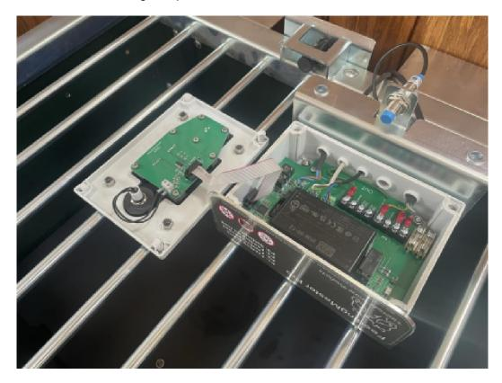
[ ] Remove the plug from the connector labeled "Motor".
