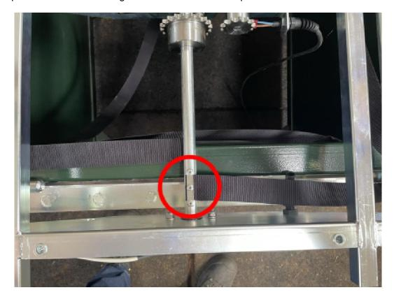
[ ] Hold the drive shaft to prevent it from rotating when installing the chain. Place the chain with one link in the top tooth of the large sprocket on the drive shaft.
