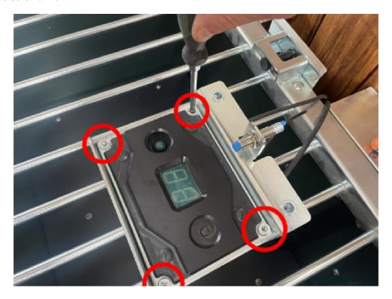
**WARNING**: If the nuts are tightened too hard, the silicone gasket between the front and back of the housing will be crushed and the two parts will no longer be watertight. Moisture can then condense in the housing, causing the controller to malfunction.
