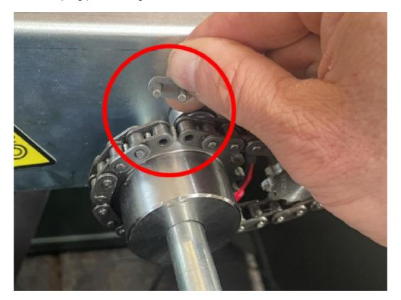
[ ] Place the retaining plate over the coupling part.
