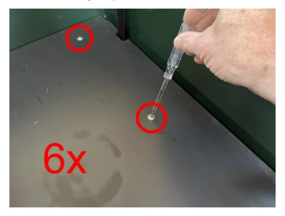
[ ] Unscrew the 6 allen bolts from the feed floor with a 4mm allen key.
