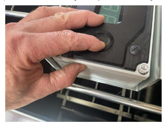
[ ] Secure the front of the housing by lightly tightening one of the nuts.
