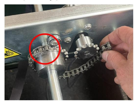
[ ] Hold the drive shaft to prevent it from rotating when installing the chain. Pull the chain around the motor sprocket and place the end in the tooth next to the top tooth of the large sprocket.
