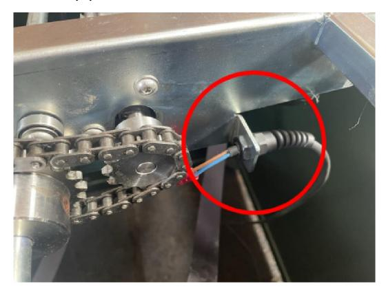
[ ] Rotate the drive shaft so that the suspension straps are completely unwound. The suspension strap closest to the blue height sensor should be on top of the drive shaft.
