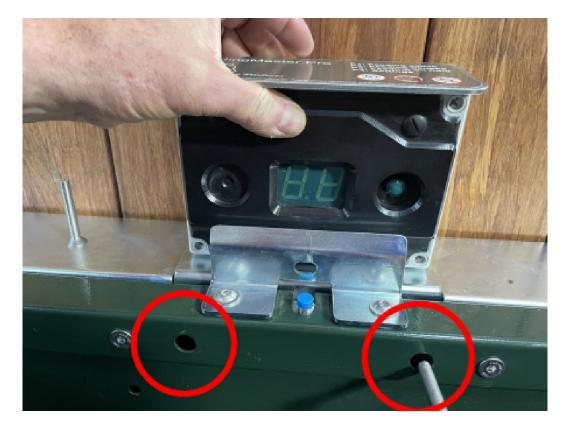
[ ] Slowly pull the wires of the motor and the height sensor as far as possible into the FeedingMaster Pro.
