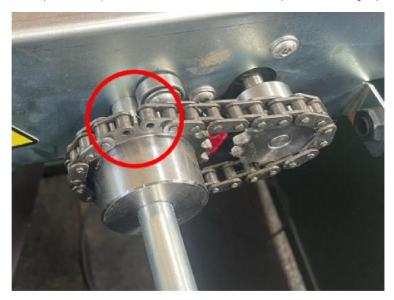
[ ] Slide the coupling piece through both ends of the chain.
