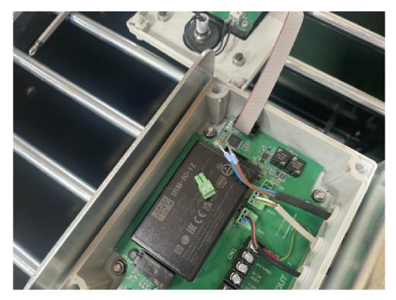
[ ] Unscrew the last part of the strain relief at the rear of the controller unit that feeds the motor cable into the controller unit. Remove the cable from the strain relief. Place the loosened part of the strain relief back half a turn so that it is not forgotten later.
