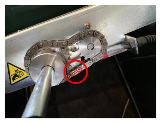
[ ] Using needle-nose pliers, squeeze the retaining clip backwards.
