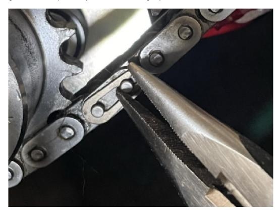
[ ] Remove the retaining clip from the retaining plate.
