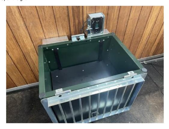
[ ] Grab the controller and tilt it forward. Lower the controller between the mounting brackets. Hook the grid sensor into the recess under the grid closure bracket.
