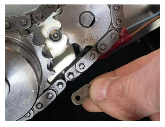
[ ] Remove the coupling part from the chain. Hold the feed mechanism securely so that it does not fall once the chain has been released.
