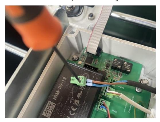
[] Remove the wires from the plug.
