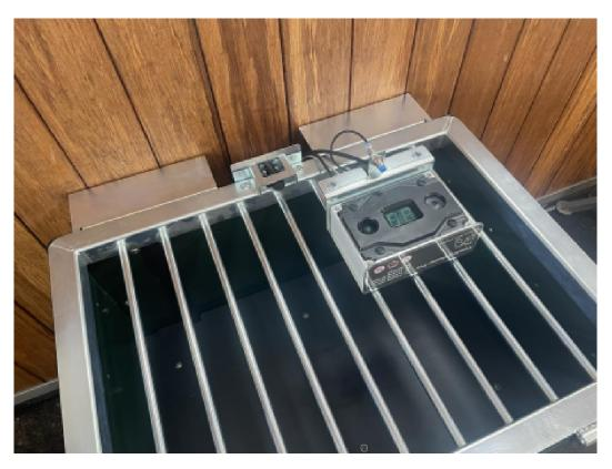
[] Unscrew the 4 bolts from the front of the controller housing with a Phillips screwdriver. The bolts are secured to the front of the housing. These can only be unscrewed, but not removed.
