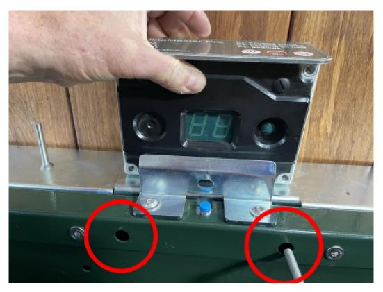
[] Close the grid and switch on the mains voltage of the FeedingMaster Pro again. Check the correct operation of the grid sensor by opening the grid. The feed floor of the FeedingMaster Pro must then be lowered to the filling position.
