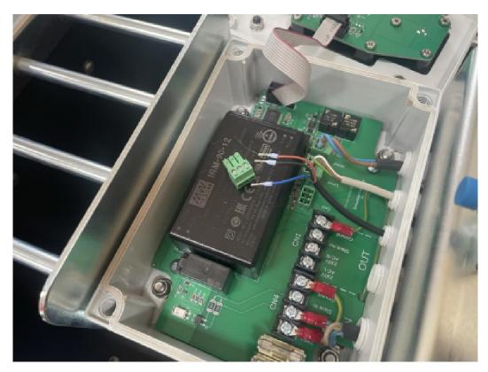
[] Unscrew the last part of the strain relief on the back of the controller unit that feeds the cable from the grid sensor into the controller unit. Remove the grid sensor cable from the strain relief. Place the loosened part of the strain relief back half a turn so that it is not forgotten later.
