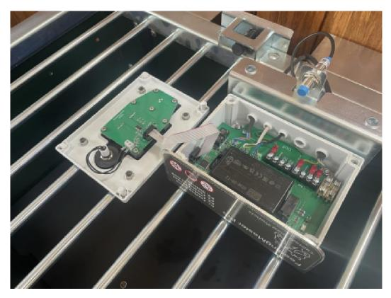
[] Remove the plug from the connector labeled "Grid".
