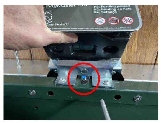
[] Tilt the controller back. Secure the controller with two M8x60 countersunk bolts.
