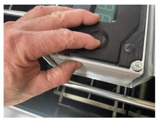
[] Secure the front of the housing by finger-tightening the four nuts. Tighten the nuts 1/8 turn of the screwdriver.
