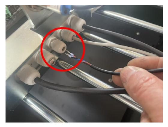
[] Place the wires in the plug and screw it hand tight. Check whether the colors of the wires are connected correctly. Then tighten them 1/8 to 1/4 turn of the screwdriver.
