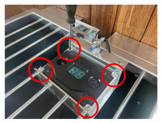
[] Lift the front of the housing and place it to the left of the controller.
