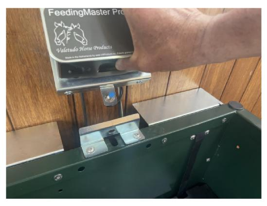
[] Tilt the controller 90 degrees clockwise and place it on the right mounting bracket.
